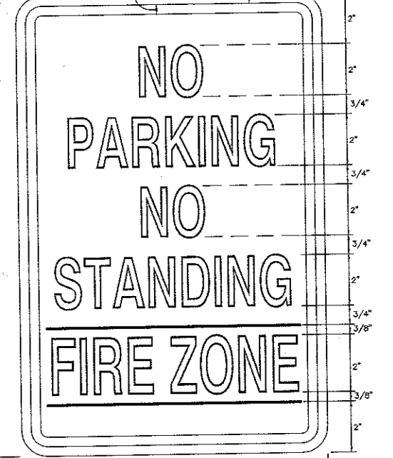
LETTERING AND BORDER RED BACKGROUND WHITE SIGN FOR FIRE LANES N.T.S. SEPARATION 100 FT. (4)
